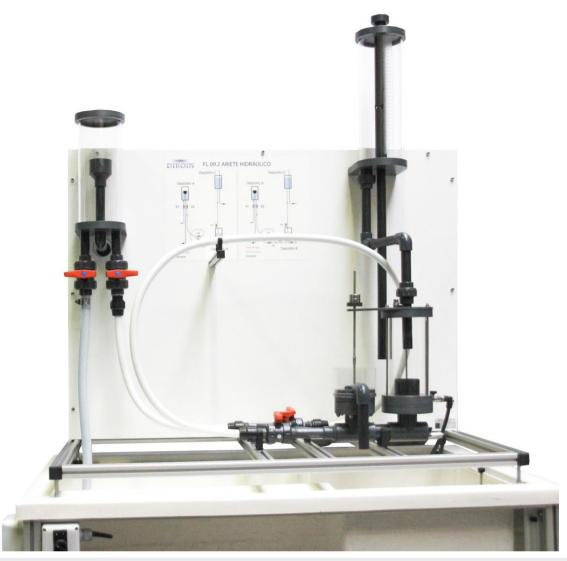
The FL09.2 is a equipment that aims to demonstrate and study the phenomenon known as water hammer, this phenomenon is the one that occurs due to the rapid closure of the passage of water through a pipe. The design of the equipment is made with special emphasis on the didactic field, so it is supplied with variable elements, to achieve a greater number of tests for a better understanding of the student.
